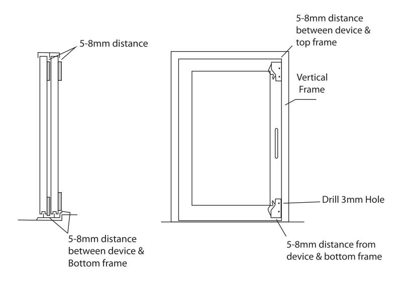
To fit Tiger, close the sliding door well. Place the long side of the Tiger against the vertical frame. Leave 5-8mm on the top or bottom horizontal frames for the teeth to engage.
